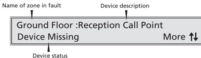
For device specific faults, pressing the **more information** again will display the unique ID code and address location of the faulty device for the benefit of service engineers, etc.
