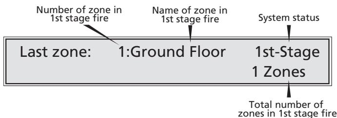
If the 1st-Stage alarm is in a zone set up with a zone dependency function:-
