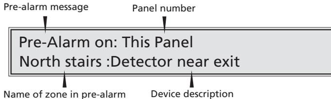
Should there be more than one detector in pre-alarm, the top right hand corner of the display will read '**More.** ↑↓' and can be scrolled through using the panel's ▲ or ▼ buttons
