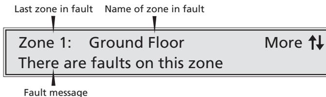
Should there be more than one fault condition, the top right side of the display will read '**More.** ↑↓' and you can scroll through them using the panel's ▲ or ▼ buttons.
