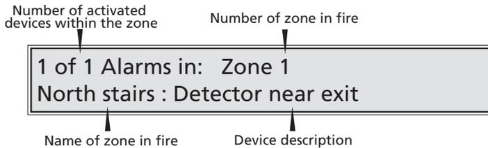
If more than one device is in a fire condition on the zone, the top left corner of the display will show, for example "1 of 3" and can be scrolled through using the ▲ and ▼ buttons.
