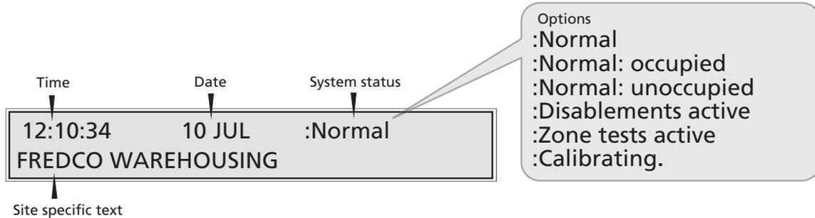
**Normal** is displayed when there are no fires, faults or pre-alarms on the system and the panel's day/night (building occupied/unoccupied) facility HAS NOT been set up by the system engineer.
